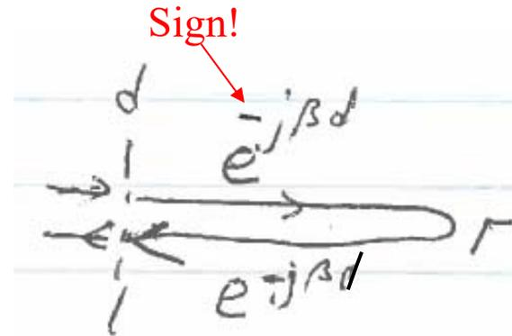
$\Gamma_d$  is just phase-shifted by  $-2\beta d$  from  $\Gamma$ .
