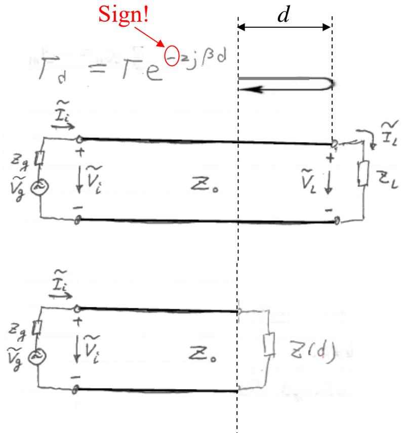
Insert  $\begin{cases} \Gamma = \Gamma_r + j\Gamma_i \\ z_L = r_L + jx_L \end{cases}$  into  $z_L = \frac{1 + \Gamma}{1 - \Gamma}$ , then use
