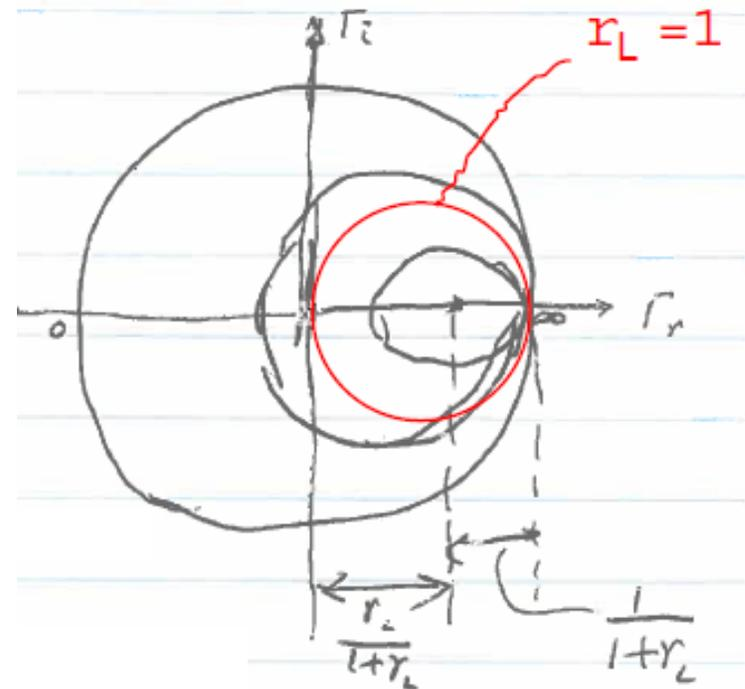
Each of these circles represent all  $\Gamma = \Gamma_r + j\Gamma_i$  that correspond to a given  $r_L$ .
